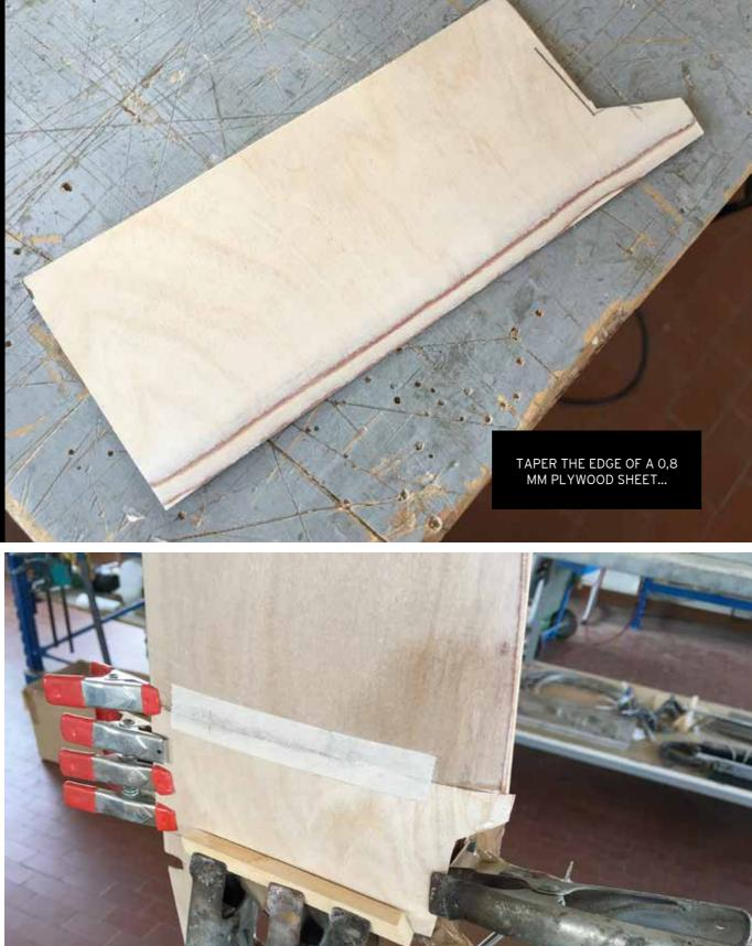
NOTE: DURING THIS GLUING BE SURE THAT THE FIN IS PERFECTLY ALIGNED WITH THE FUSELAGE
