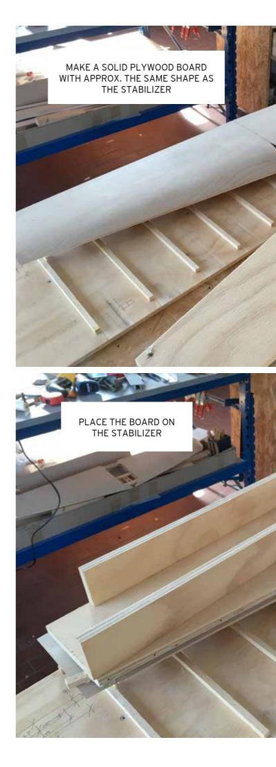
NOTE: I ADDED TWO STRIP TO REINFORCE THE BOARD, IT IS NOT NECESSARY IF THE BOARD IS STRONG ENOUGH
