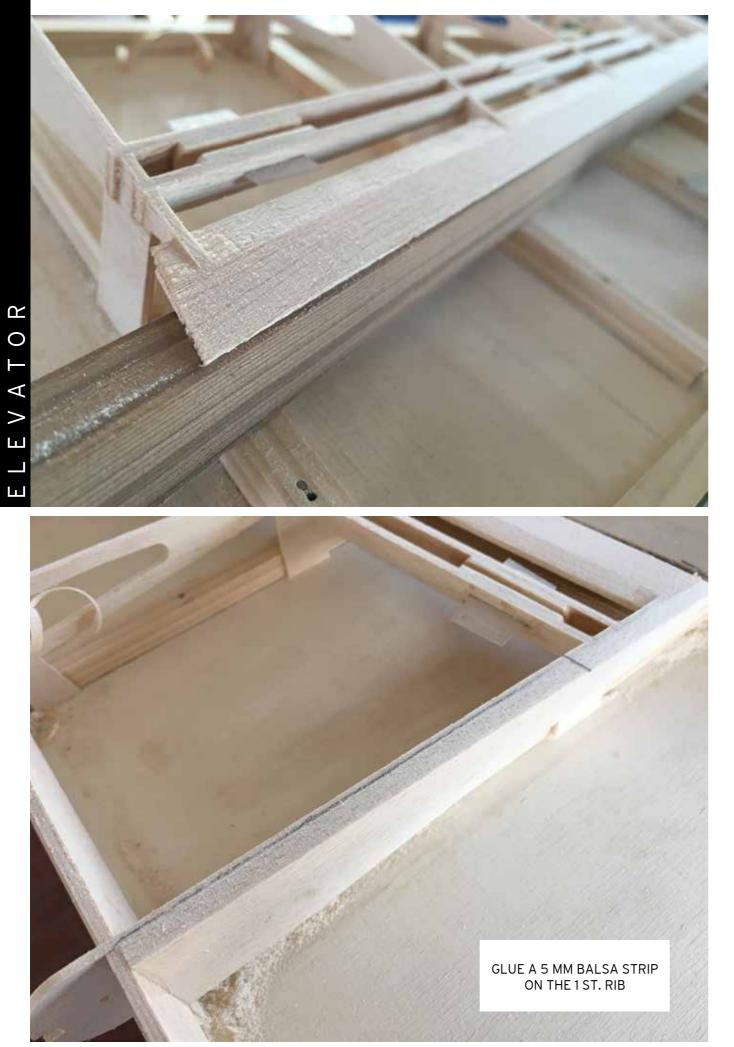
GLUE THE 0.6 MM PLYWOOD SHEETING ON THE ELEVATOR TRIM TAB AND ON THE TRAILING EDGE
