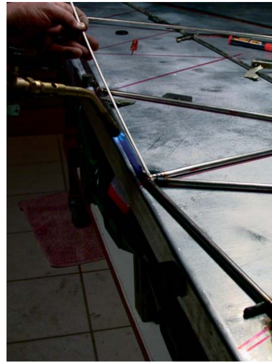
Above: the beginning stage of construction of the fuselage. The first side is welded following the drawing outlined on the metal table. The tubes are locked in position with magnets.
