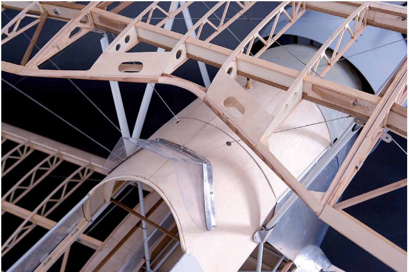
On the left: lower wing structure (the upper one is basically the same)
