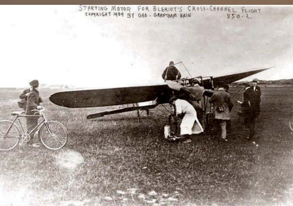
Picture on Left: Starting the Blériot before the Channel crossing. Pictures at Right: Anzani engine, 25 HP and Louis Blériot with Alessandro Anzani, designer and builder of the engine. The engine for the crossing was a 3 cylinder mounted like a 'W'. Later Anzani built radial engines with 3 cylinders, like the one used on this model.
