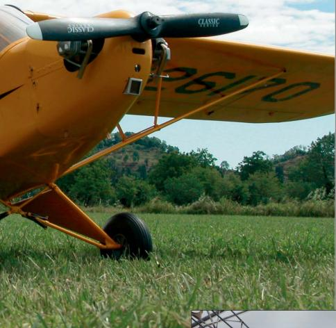
The wing consists of two halves attached to the fuselage with two alignining dowels and two turnbuckles. The struts are made of stainless ste-
