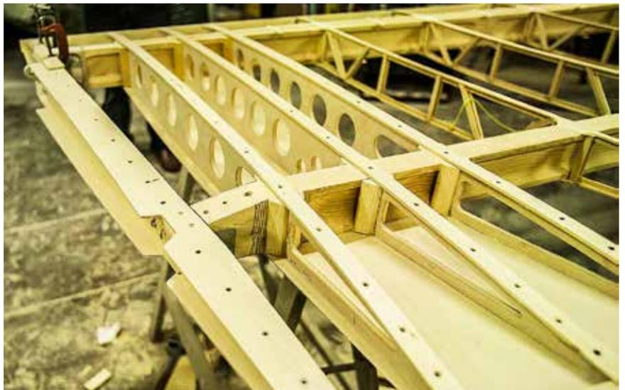
Bottom wing of a real Tiger Moth under restoration, the upper plywood sheeting is modified now to represent the original.
