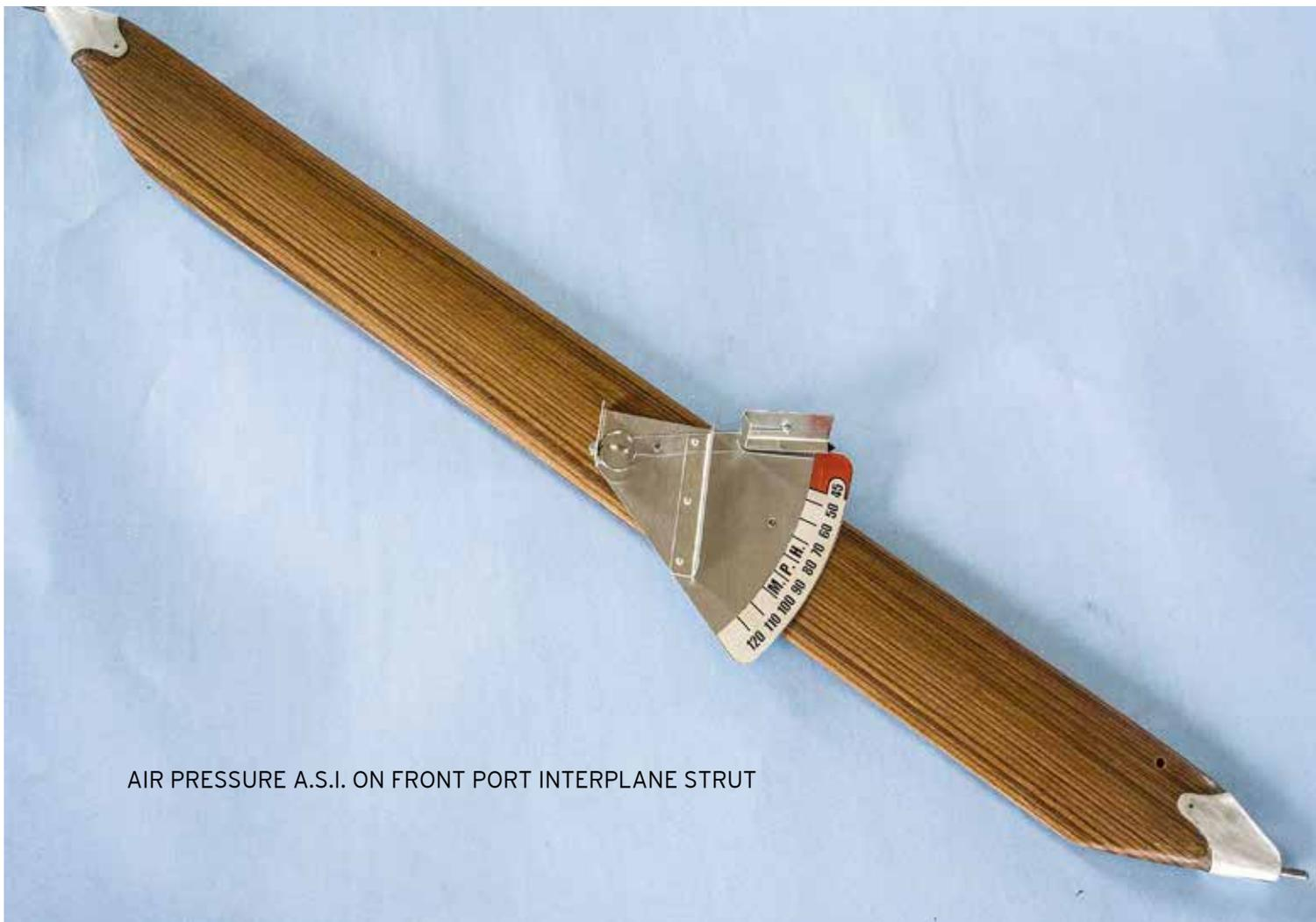
AIR PRESSURE A.S.I. ON FRONT PORT INTERPLANE STRUT
