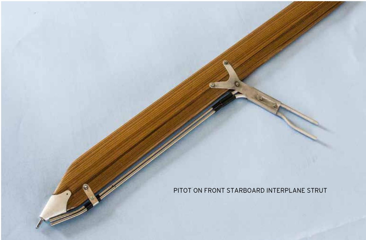
PITOT ON FRONT STARBOARD INTERPLANE STRUT
