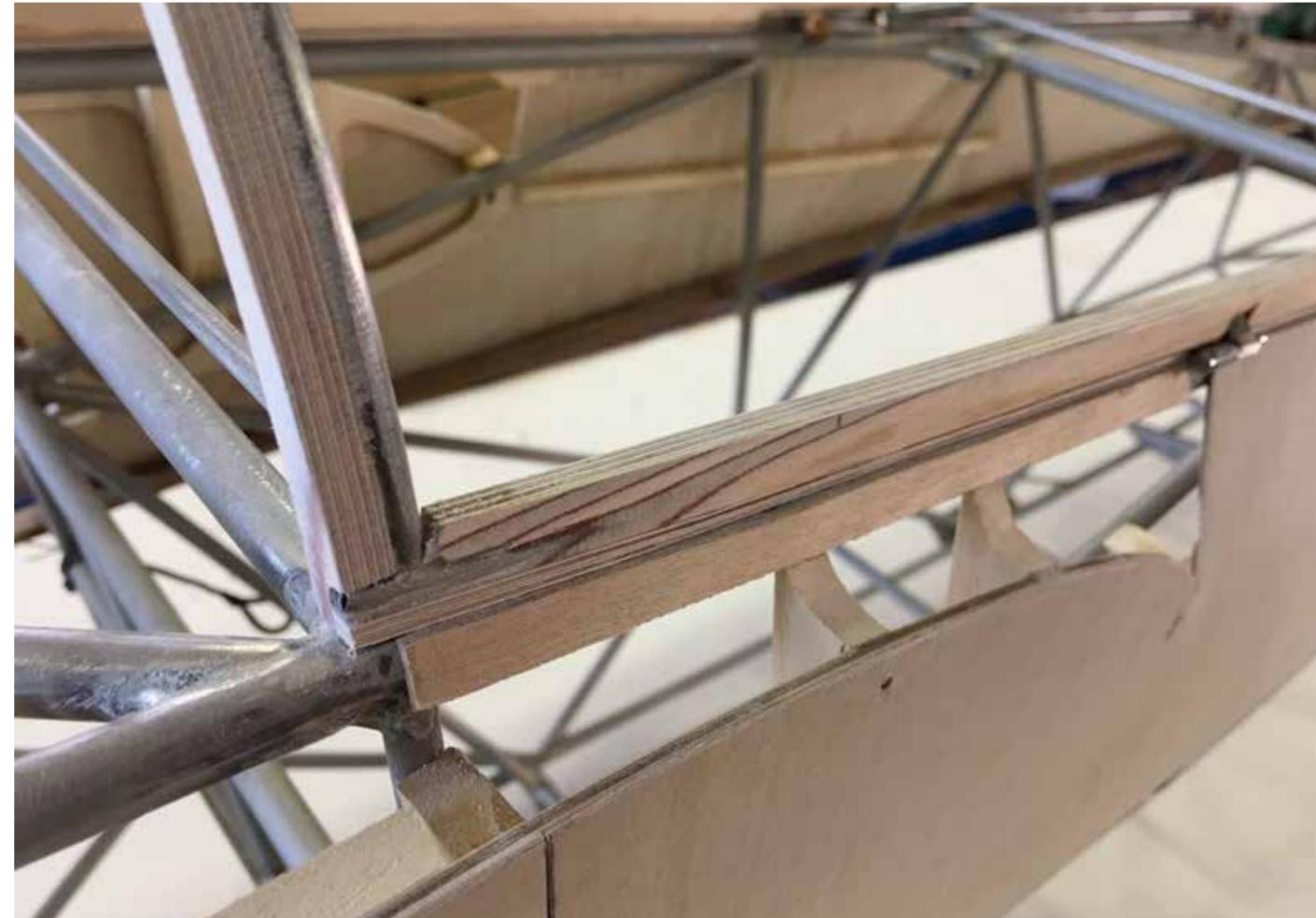
CHECK THE ALIGNMENT WITH THE 1ST. BULKHEAD, CONSIDER THAT THE CANOPY THICKNESS IS APPROX. THE SAME AS THE PLYWOOD COVERING
