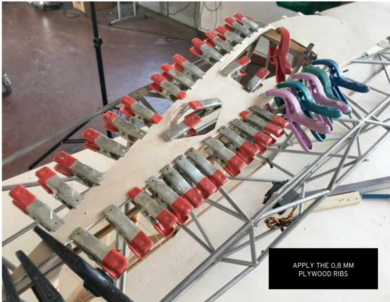
APPLY THE 0.8 MM PLYWOOD RIBS
