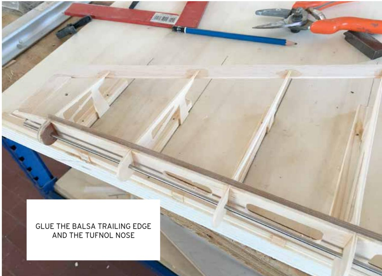
GLUE THE Balsa TRAILING EDGE AND THE TUFNOL NOSE
