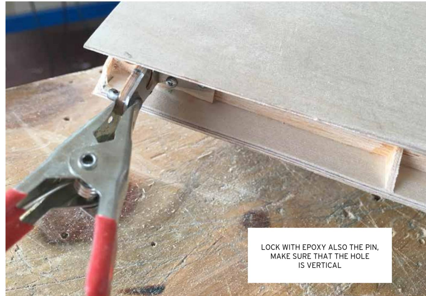
LOCK WITH EPOXY ALSO THE PIN, MAKE SURE THAT THE HOLE IS VERTICAL
