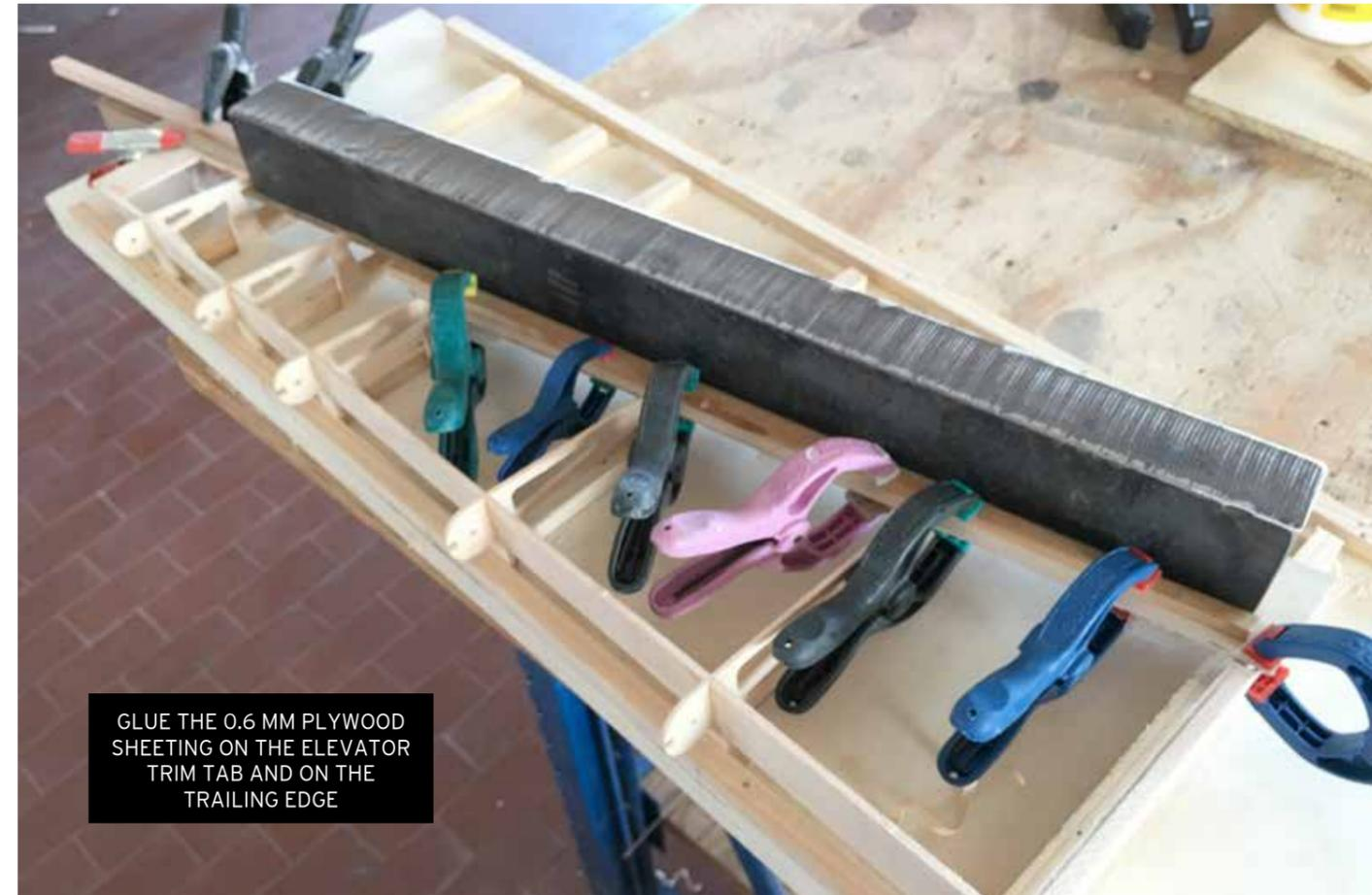
GLUE THE 0.6 MM PLYWOOD SHEETING ON THE ELEVATOR TRIM TAB AND ON THE TRAILING EDGE
