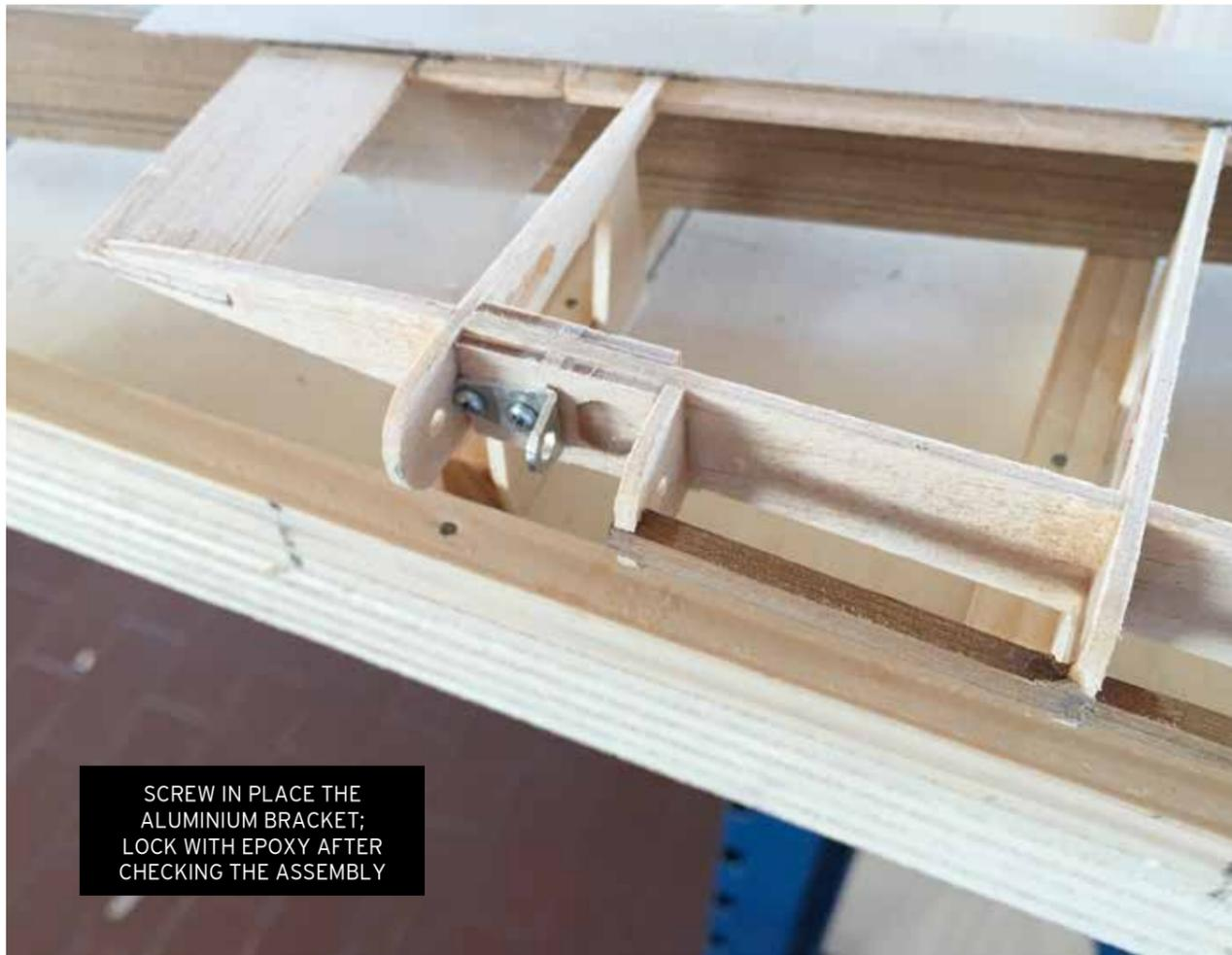
SCREW IN PLACE THE ALUMINIUM BRACKET; LOCK WITH EPOXY AFTER CHECKING THE ASSEMBLY
