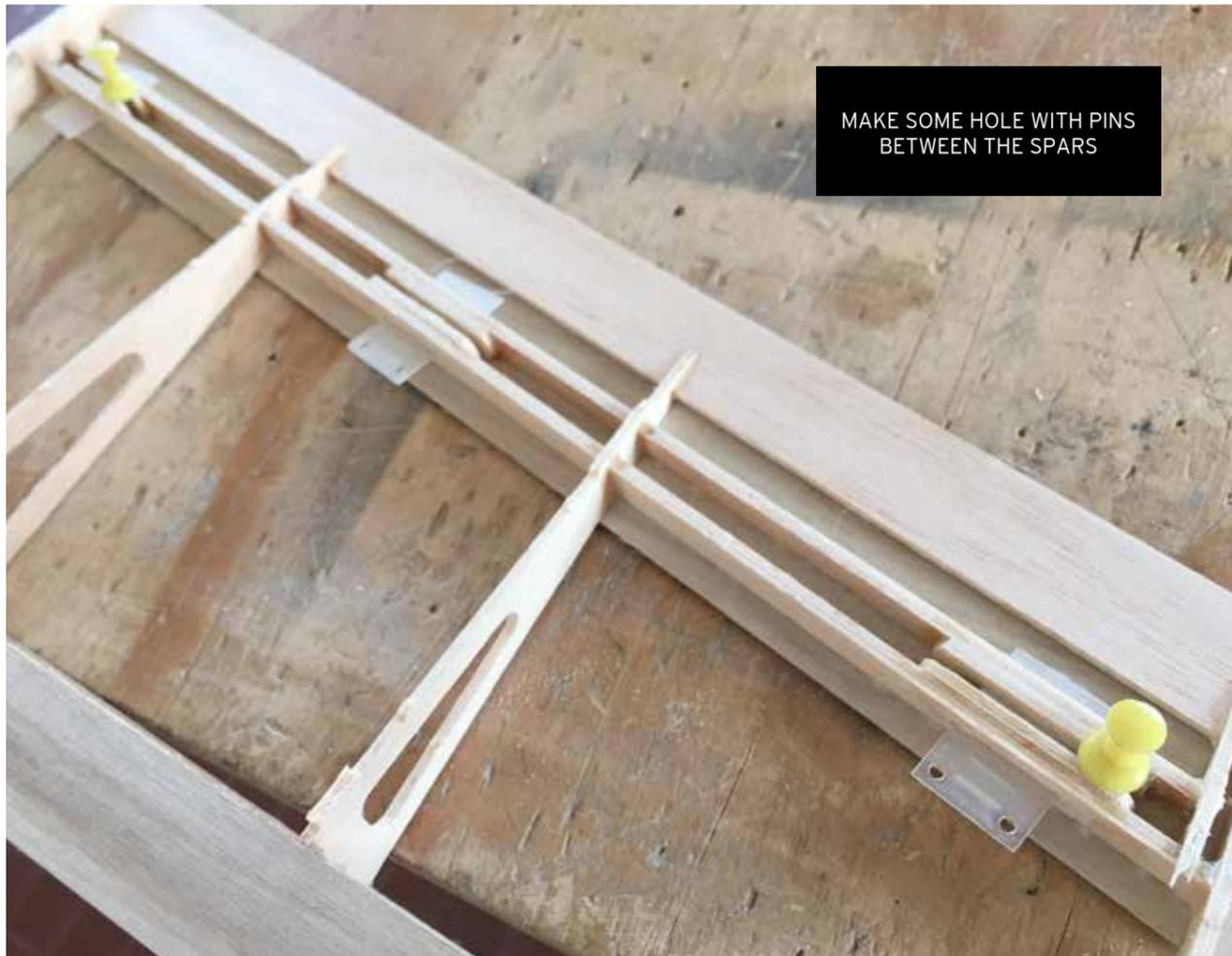
MAKE SOME HOLE WITH PINS BETWEEN THE SPARS
