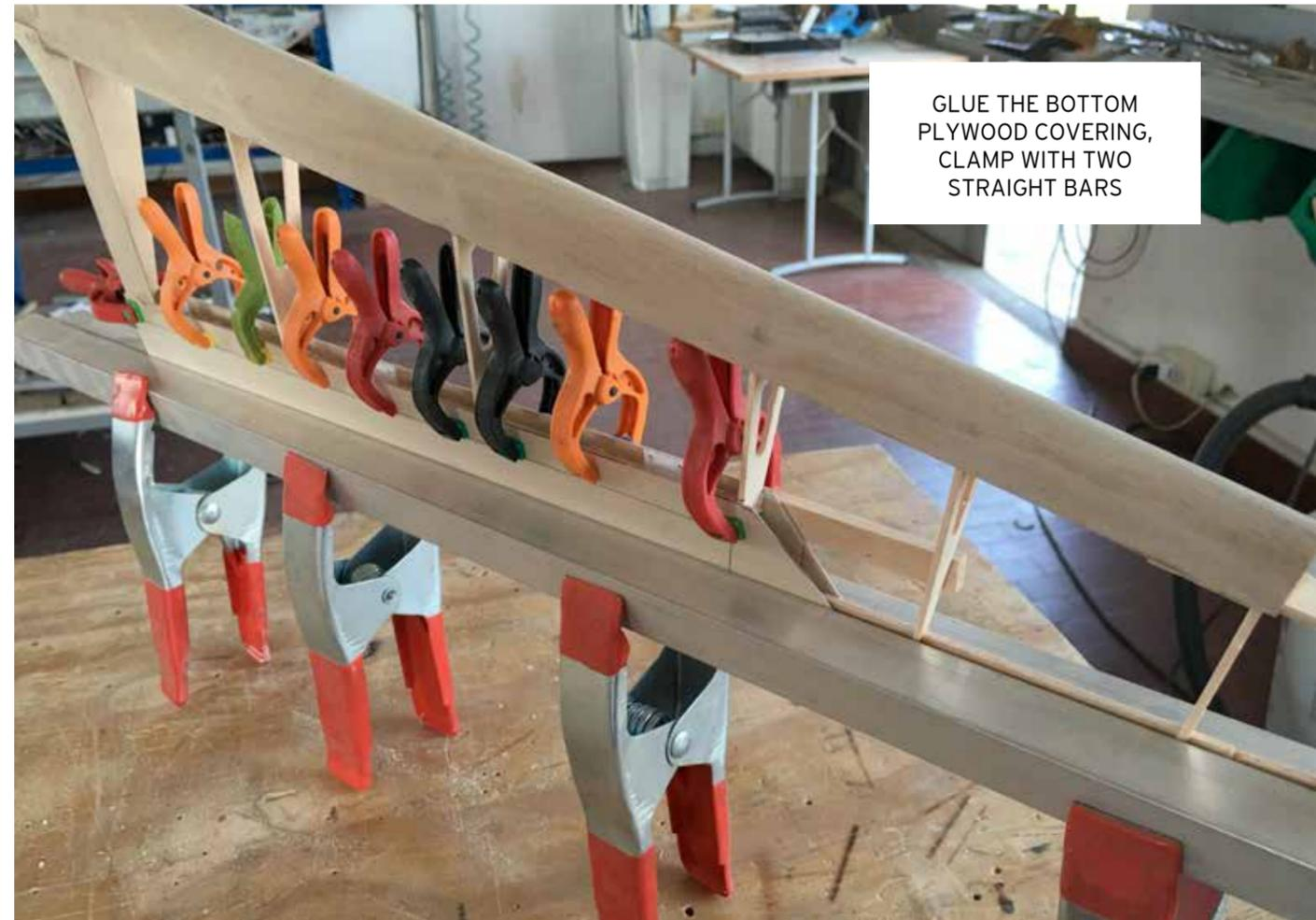
GLUE THE BOTTOM PLYWOOD COVERING, CLAMP WITH TWO STRAIGHT BARS
