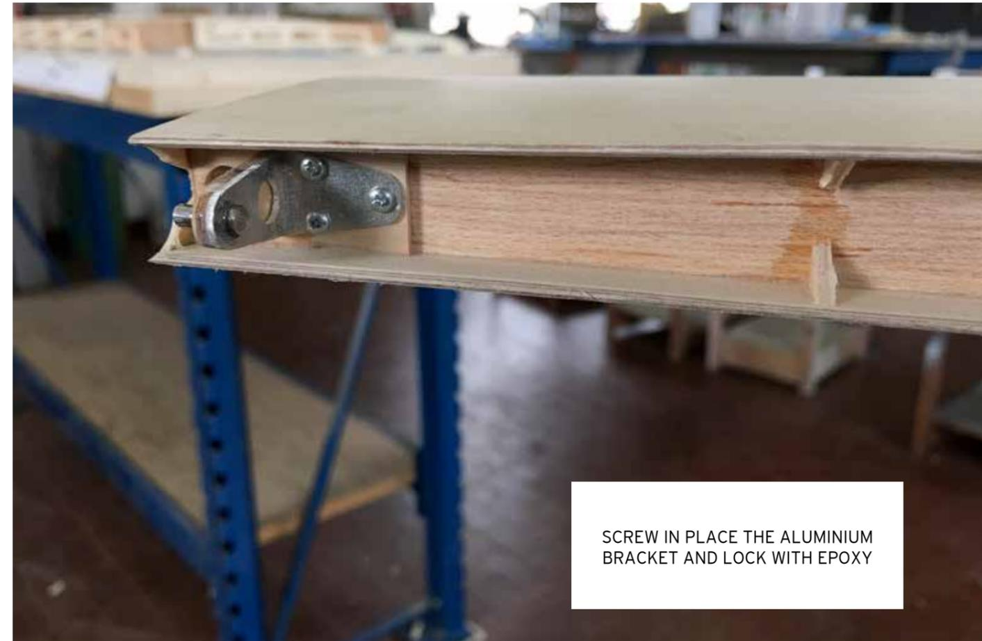
SCREW IN PLACE THE ALUMINIUM BRACKET AND LOCK WITH EPOXY
