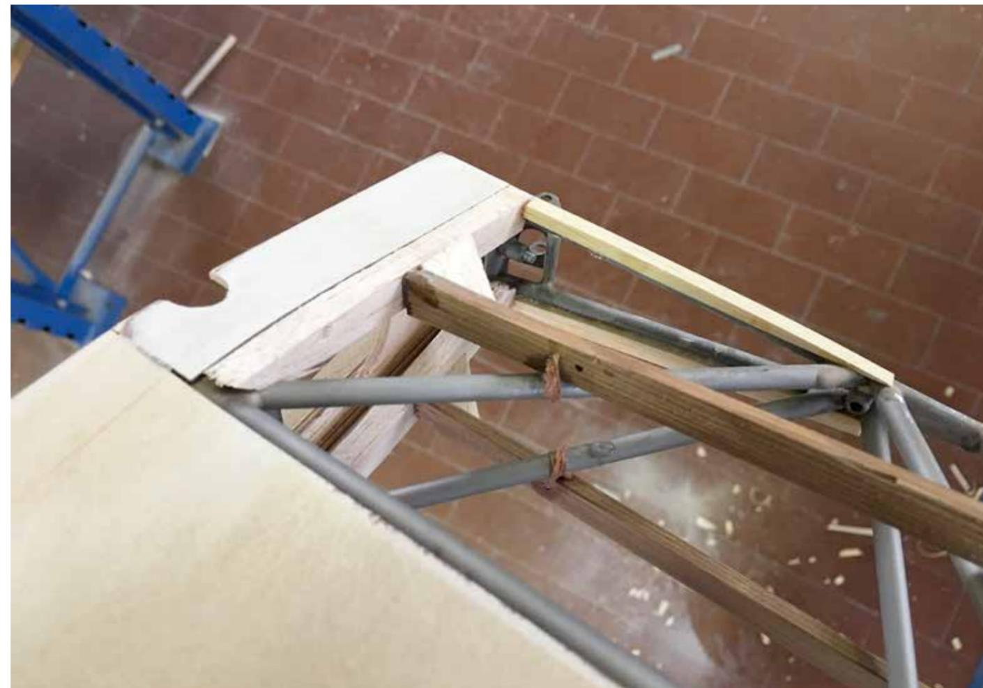
AS FOR THE RUDDER, USE THE FRAME P8 TO MARK THE RIBS POSITION AND NAIL SOME STRIPS 10 x 10 TO THE BUILDING BOARD, THEN GLUE THE RIBS TO THE STRIPS
