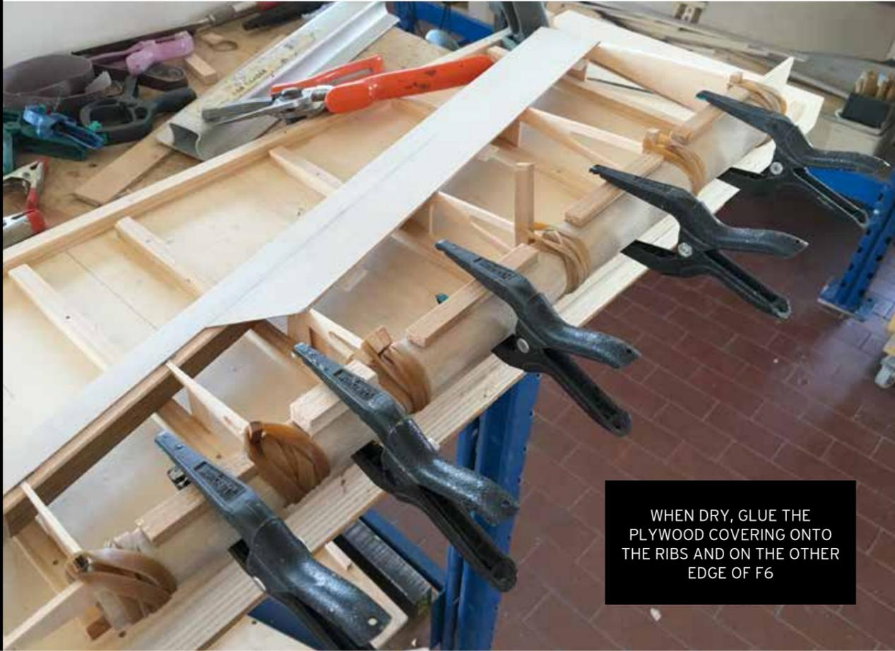
WHEN DRY, GLUE THE PLYWOOD COVERING ONTO THE RIBS AND ON THE OTHER EDGE OF F6
