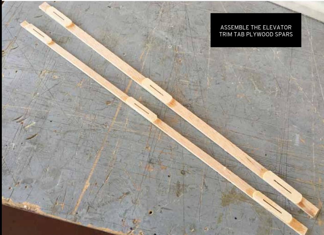
ASSEMBLE THE ELEVATOR TRIM TAB PLYWOOD SPARS
