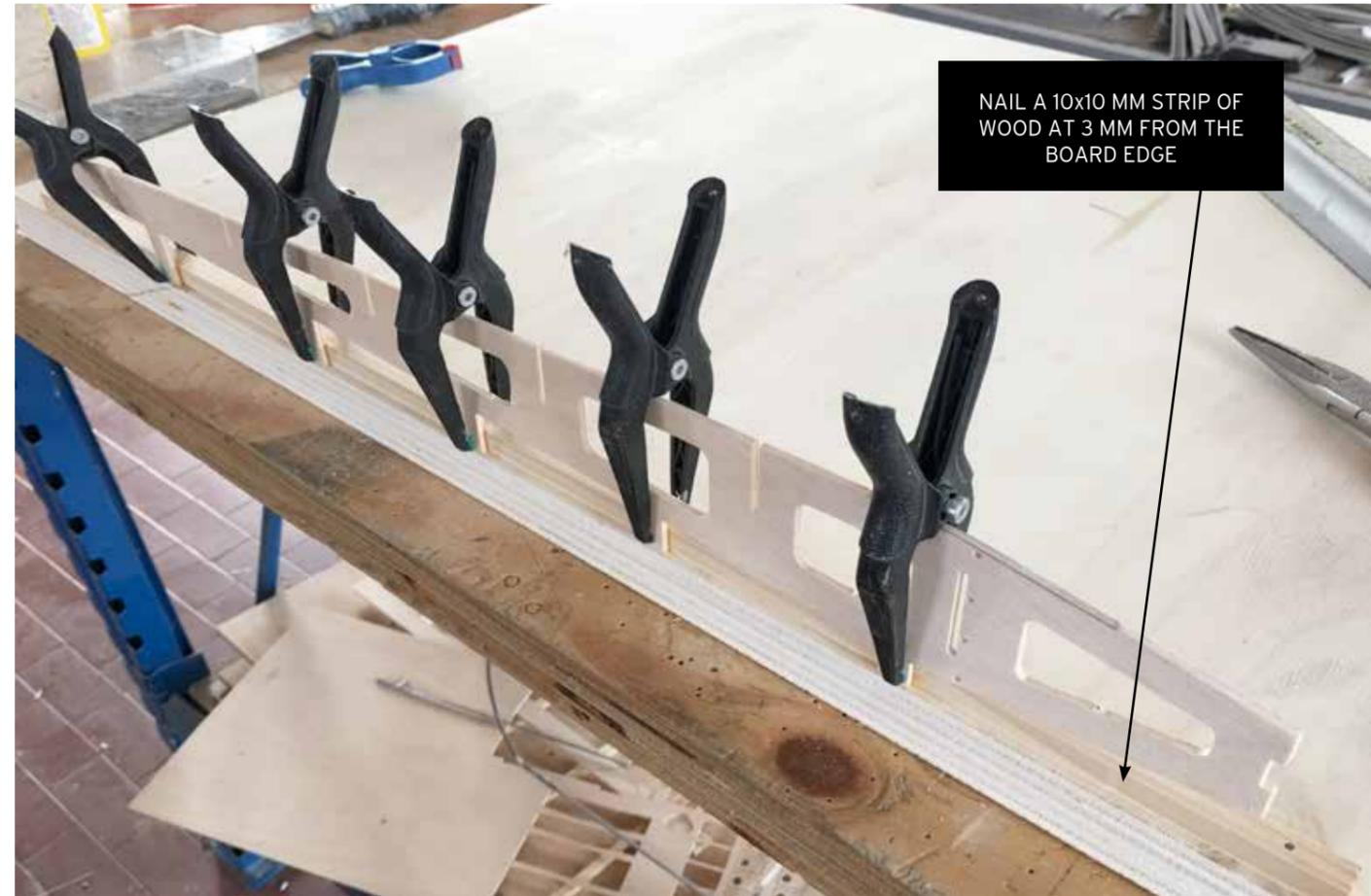
NAIL A 10x10 MM STRIP OF WOOD AT 3 MM FROM THE BOARD EDGE
