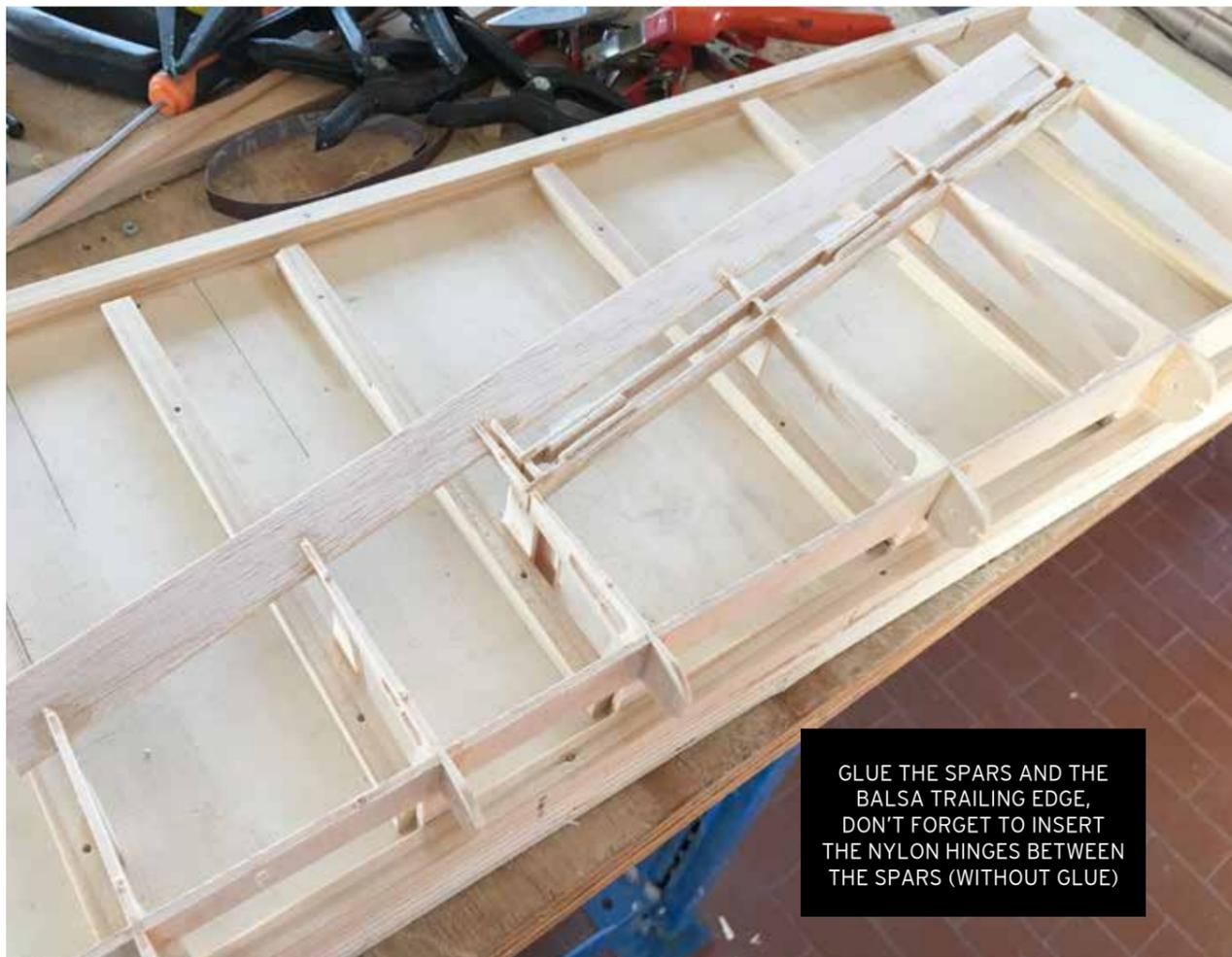
GLUE THE SPARS AND THE Balsa TRAILING EDGE, DON'T FORGET TO INSERT THE NYLON HINGES BETWEEN THE SPARS (WITHOUT GLUE)
