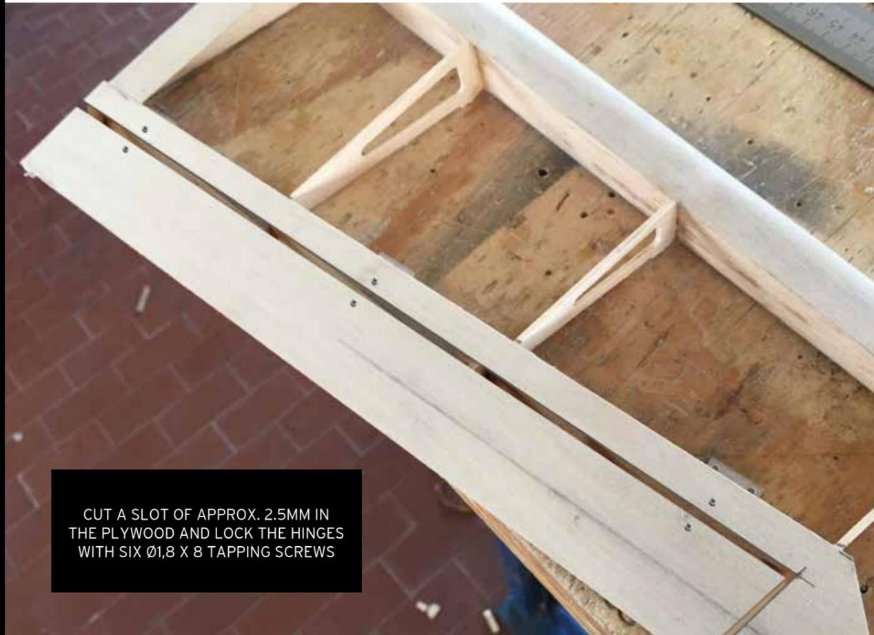
CUT A SLOT OF APPROX. 2.5MM IN THE PLYWOOD AND LOCK THE HINGES WITH SIX Ø1,8 X 8 TAPPING SCREWS
