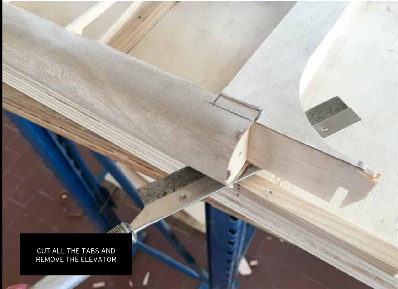
CUT ALL THE TABS AND REMOVE THE ELEVATOR
