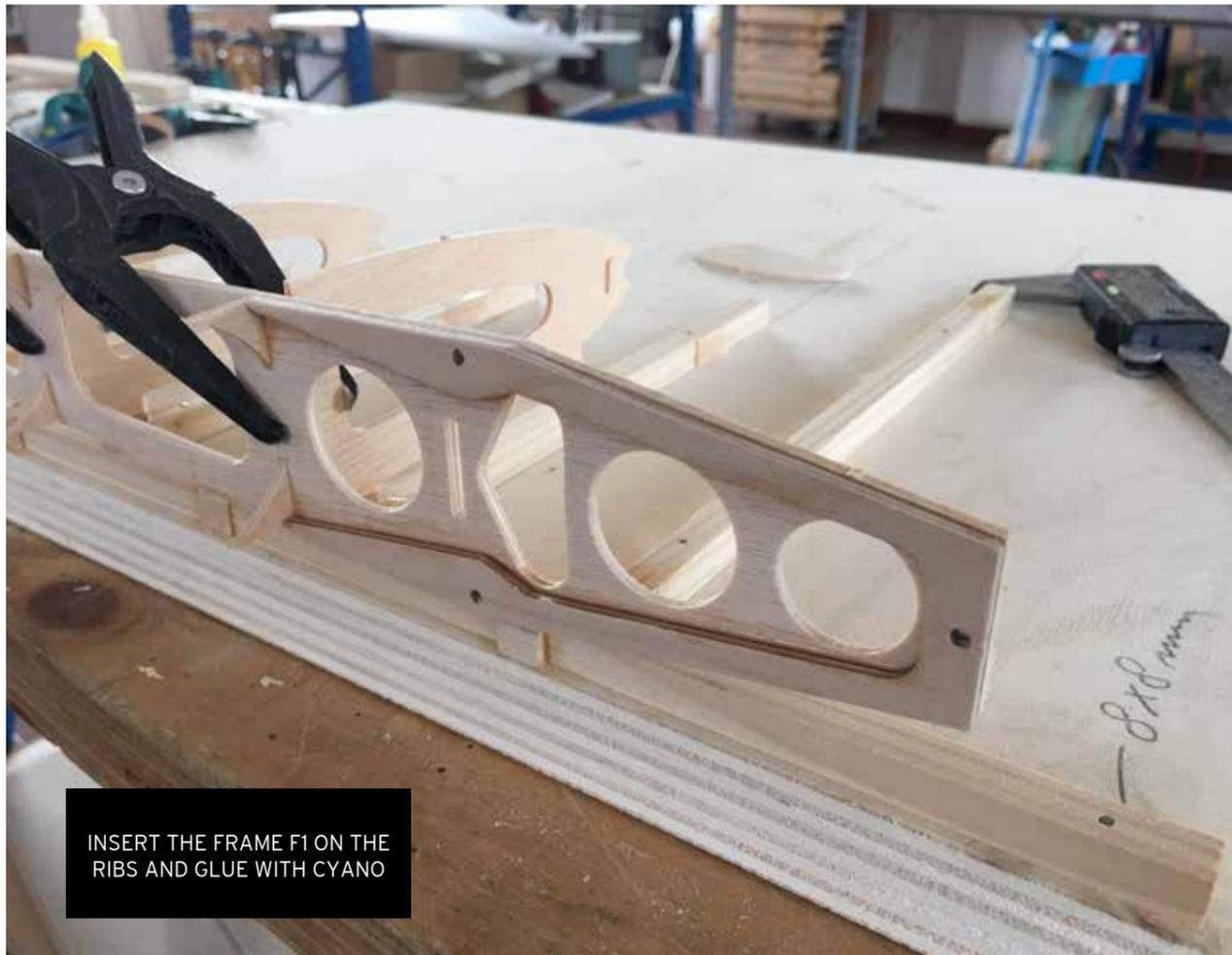
INSERT THE FRAME F1 ON THE RIBS AND GLUE WITH CYANO
