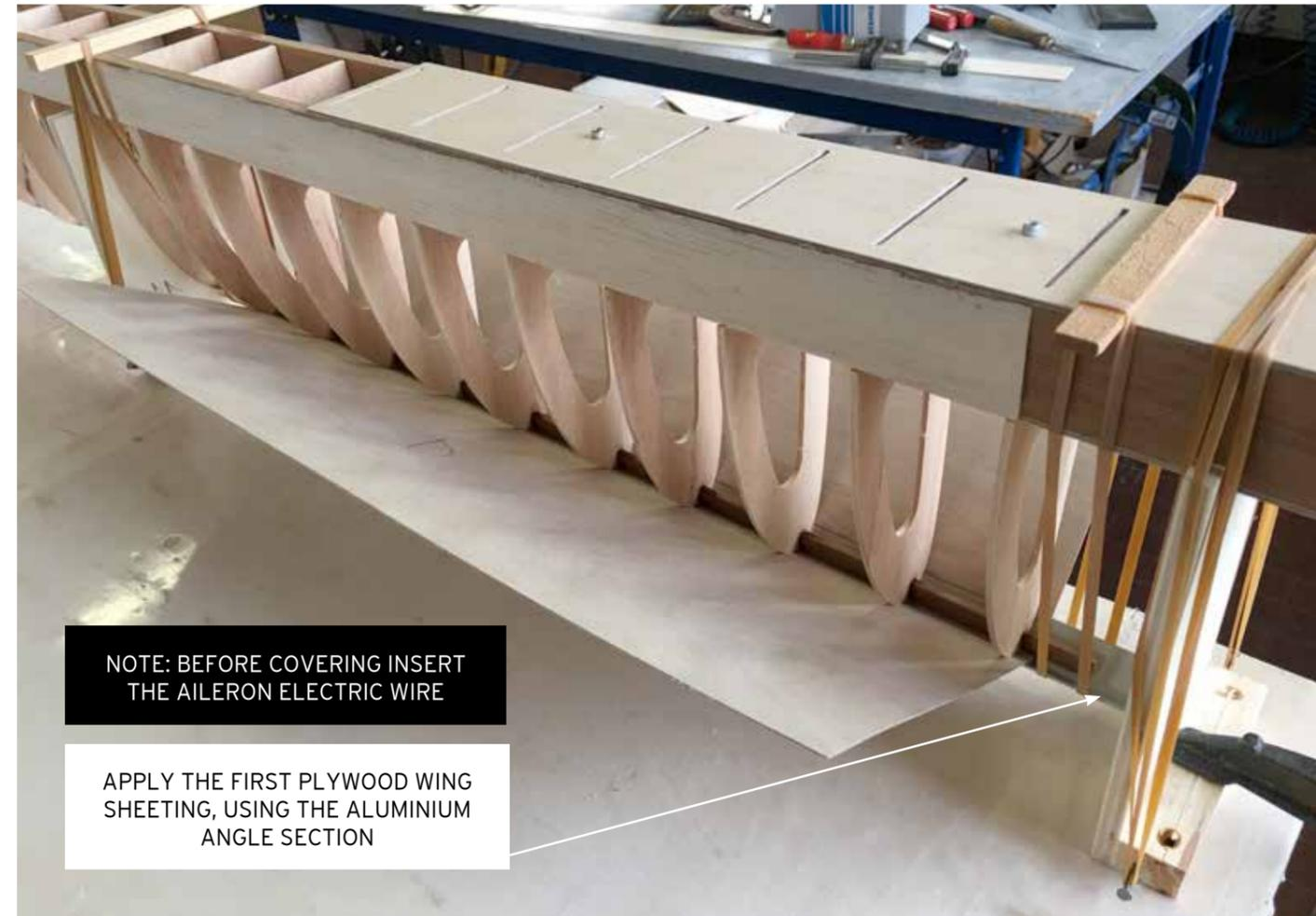
NOTE: BEFORE COVERING INSERT THE AILERON ELECTRIC WIRE
