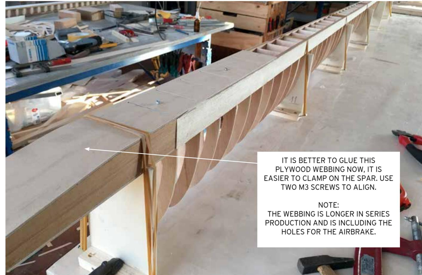
IT IS BETTER TO GLUE THIS PLYWOOD WEBBING NOW, IT IS EASIER TO CLAMP ON THE SPAR. USE TWO M3 SCREWS TO ALIGN.
