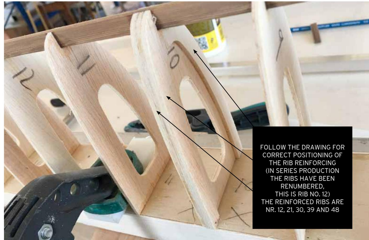
FOLLOW THE DRAWING FOR CORRECT POSITIONING OF THE RIB REINFORCING (IN SERIES PRODUCTION THE RIBS HAVE BEEN RENUMBERED, THIS IS RIB NO. 12) THE REINFORCED RIBS ARE NR. 12, 21, 30, 39 AND 48
