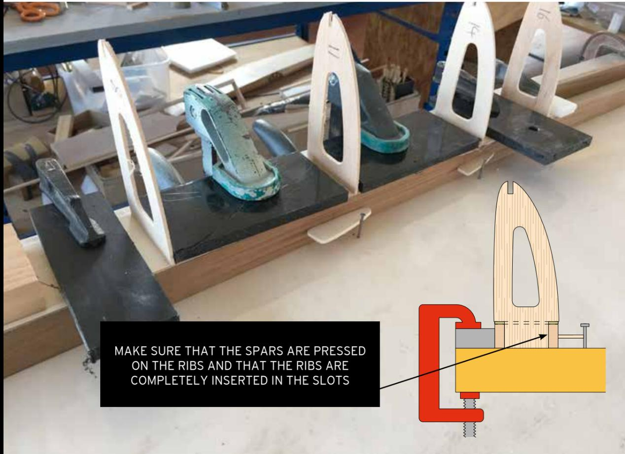
MAKE SURE THAT THE SPARS ARE PRESSED ON THE RIBS AND THAT THE RIBS ARE COMPLETELY INSERTED IN THE SLOTS
