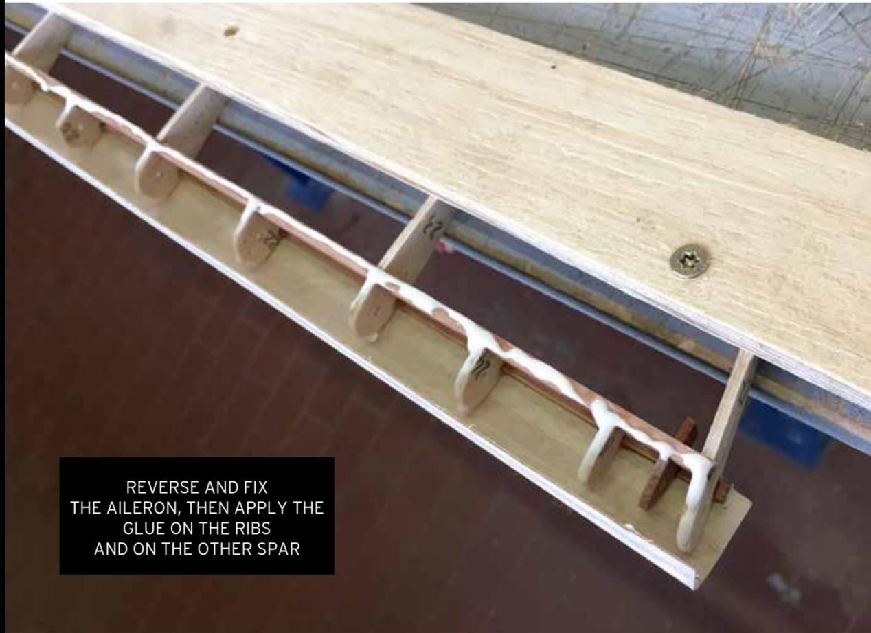
REVERSE AND FIX THE AILERON, THEN APPLY THE GLUE ON THE RIBS AND ON THE OTHER SPAR
