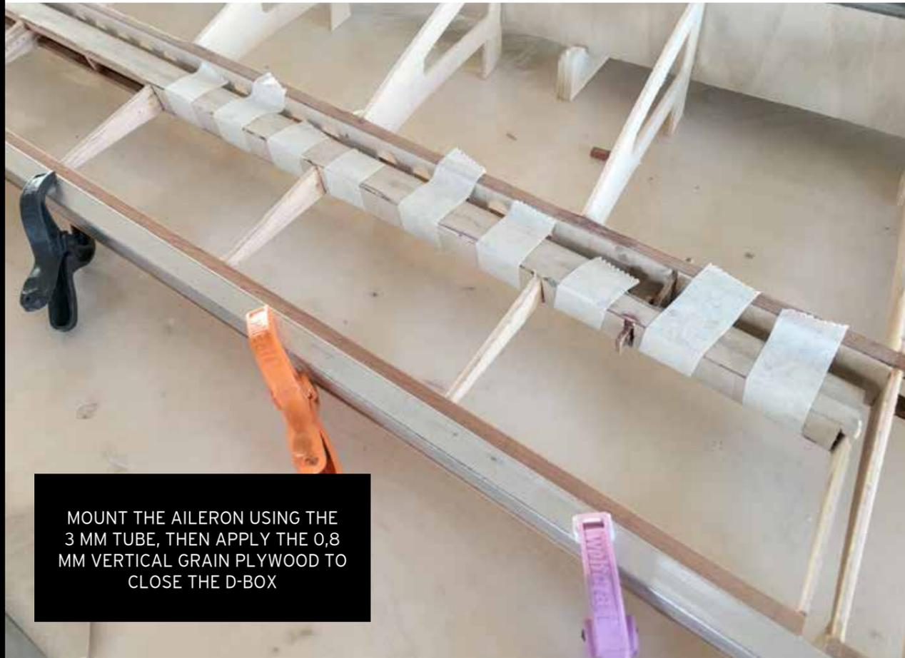
MOUNT THE AILERON USING THE 3 MM TUBE, THEN APPLY THE 0,8 MM VERTICAL GRAIN PLYWOOD TO CLOSE THE D-BOX
